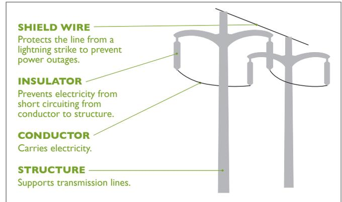
A DC transmission line has two conductor bundles called “poles.” Conductors are the wires that hang from the towers and are often bundled in groups of two or three. Like a car battery, the two bundles of DC conductors have opposite polarity, one positive and one negative. The voltage of a DC transmission line, therefore, is usually referred to as  $\pm$  (plus-minus) voltage. For example, a 500 kilovolt (kV) DC transmission line is referred to as a  $\pm 500$  kV DC transmission line.
