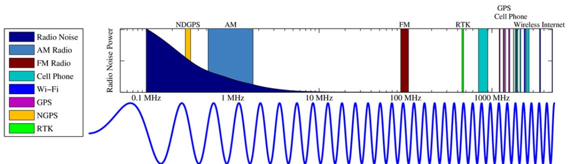
Figure 1. Magnitude of corona-generated radio noise and frequency range of various technology
